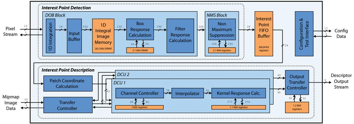
Fig. 3. ASIC Top-Level Diagram with two Descriptor Calculation Units (DCUs): The ASIC is supplied with raw 8 bit gray-scale image pixels. It first searches interest points within the image, whose surroundings are described in a second step. For the description an image patch around the interest point is transferred to the ASIC as well. The final descriptors are sent back to the FPGA for matching.
