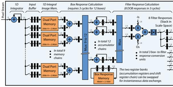
Fig. 5. The DOB filter block receives a dense pixel stream and calculates the DOB responses, which are output as stacks of eight values in scale-space (highlighted in red in Figure 4c). The constants  $I_n$  and  $O_n$  are the appropriate normalization factors for the inner and outer boxes of scale  $n$ .
