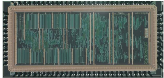
Fig. 8. Microphotograph of the SANDSTORM chip.
