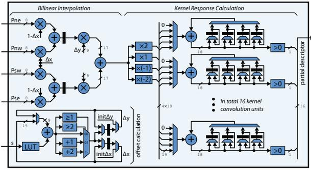
Fig. 7. The descriptor calculation unit (shown without the channel controller) contains a bilinear interpolator and 16 kernel response units. Note that the kernel weights are implemented without multipliers.
