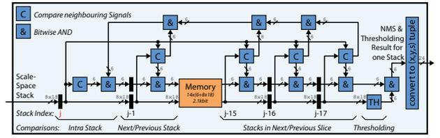
Fig. 6. The NMS block receives a stack of 8 DOB responses per pixel position (red stack in Figure 4c), performs the NMS, and applies the weak response threshold. The 8 DOB responses are stored in  $8 \times 18$  bit wide registers and the intermediate comparison results in 6 bit wide registers.
