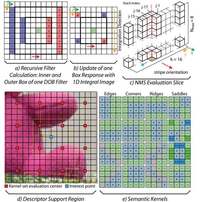
Fig. 4. Algorithmic Details: a) Recursive DOB filter calculation for the green pixel position. b) 1D integral image box response update. c) NMS evaluation: the most recently added stack is colored in red. d) The descriptor support region is overlaid over an image patch showing the centers around which the set of semantic kernels depicted in e) is evaluated.
