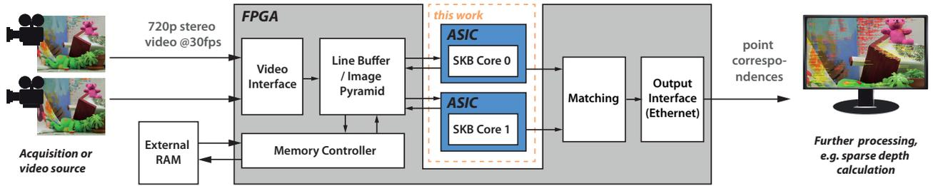
Fig. 1. Overview of the stereo video feature detection system. The FPGA (in gray) provides the IO interfaces, external memory access, and the matching operation. The ASIC (blue) performs the computationally intensive SKB feature extraction (there are two identical ASICs, one for each stereo video channel). The ‘Teddy’ image shown here is from the dataset provided by [17].
