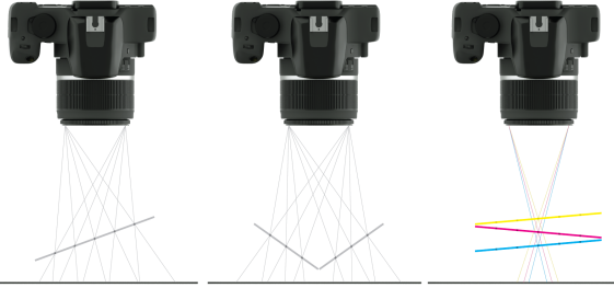
Figure 1. Sketches of the proposed setups. Left : Minimal configuration using two layers: the first layer is an emissive planar display panel and the second layer, a thin opaque sheet with a grid of holes, is placed slightly angled in front. Center : Using two tilted hole planes enables a better coverage for wide angle lenses and an additional calibration plane. Right : Three layered hole planes consisting of yellow, cyan and magenta filters allow to capture correspondences to three planes with one configuration.
