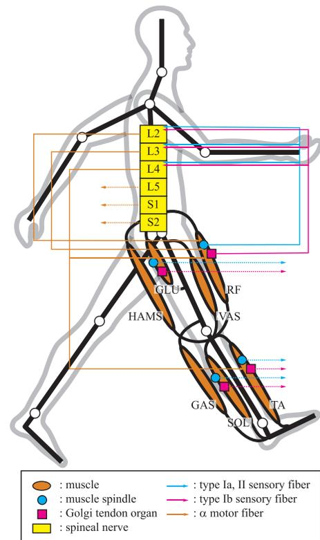
Fig. 1. The neuromusculoskeletal system. This system consists of the musculoskeletal model, physiological muscle model, proprioceptive receptor model, and neuromuscular network model. Only representative fibers and receptors are drawn.
