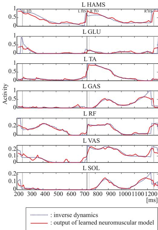
Fig. 2. The muscle activity during the walking motion. Red solid line: the output of the identified neuromusculoskeletal system, blue dotted line: the muscle activity from the dynamics computation and optimization. Black vertical solid line: L HS (left heel strike), black vertical dashed line: L TO (left toe off), gray vertical solid line: R HS (right heel strike), gray vertical dashed line: R TO (right toe off).
