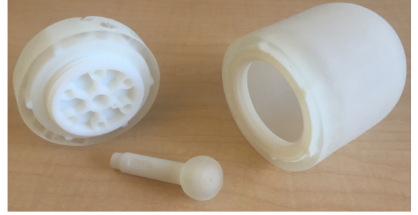
Fig. 6. 3D printed parts for soft skin module.
